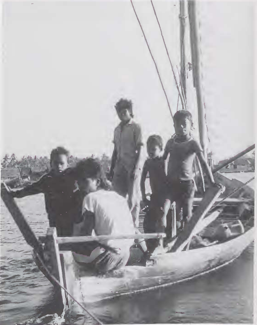
Fig. 21. The tiller is carried on the lee side of the rudder on a Mola soppe .
